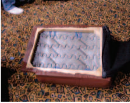
Photo 1. Seat cushion with springs that resonated at 90 Hz
